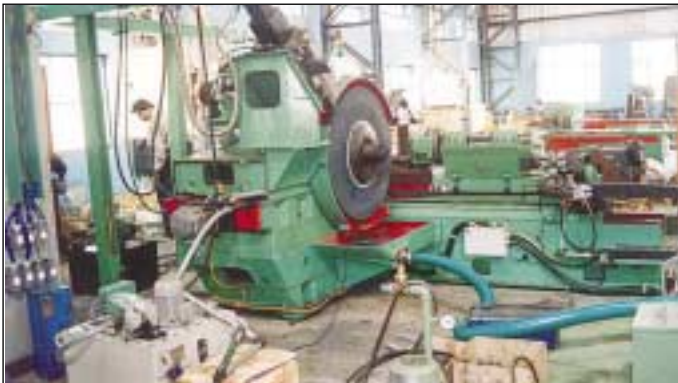
Figure 2: Nexus Union conventional crankshaft grinder after retrofitting into a CNC crankshaft grinder
