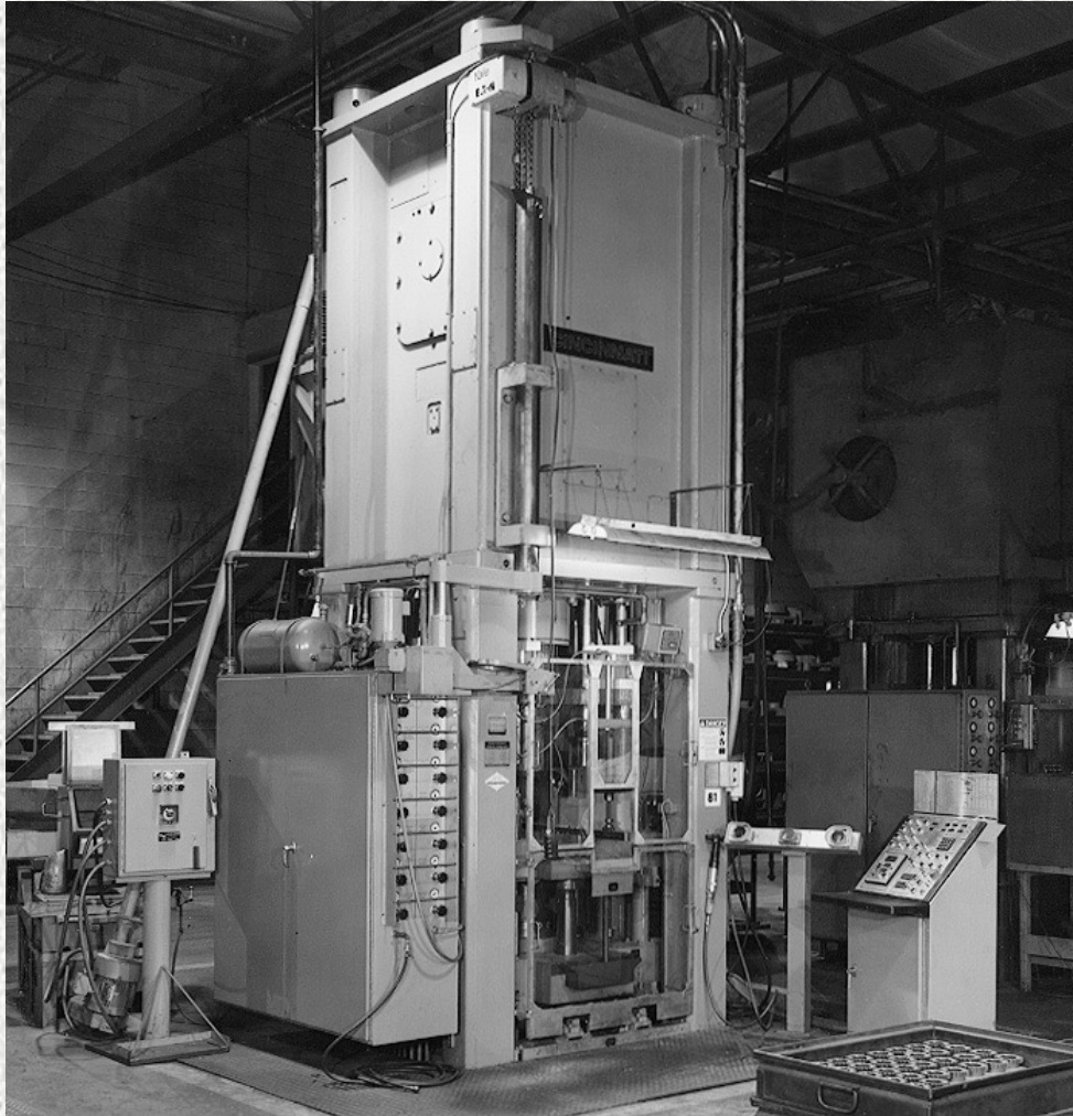
Figure 17.11 A 7.3 MN (825 ton) mechanical press for compacting metal powder. Source: Courtesy of Cincinnati Incorporated.
