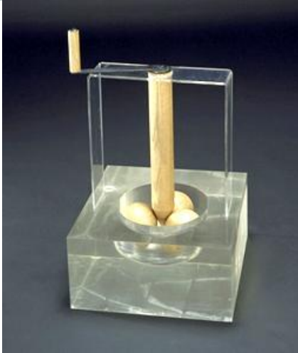
Roller and ball bearings for cone-tipped vertical axes
