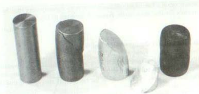
Figure 4.23 Compression specimens of metals (left to right): untested specimen, and tested specimens of gray cast iron, aluminum alloy 7075-T651, and hot-rolled AISI 1020 steel. Diameters before testing were approximately 25 mm, and lengths were 76 mm. (Photo by R. A. Simonds.)
