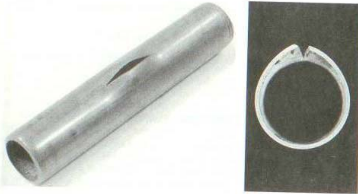
Figure 6.14 Failure of a 15 mm diameter copper water pipe due to excess pressure from freezing. In the cross section on the right, note that failure occurred on a plane inclined 45^\circ to the tube surface, which is the plane of the maximum shear stress. (Photos by R. A. Simonds.)
