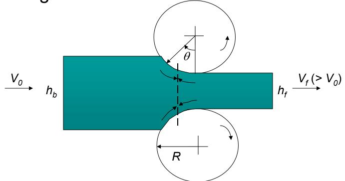
Width of plate w is large  $\rightarrow$  plane strain
