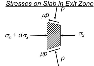
Using slab analysis we can derive roll pressure distributions for the entry and exit zones as:  $h_0$  and  $h_b$  are the same thing
