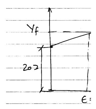
$\sigma f = Yf = 207 + 414 \epsilon$ ; Use the value of strain,  $\epsilon = 1.58$   $Yf_aver = (207 + 861)/2 = 534.06$  MPa  $Vf_aver'' = 1.15$  Vf aver and maximum value of Force
