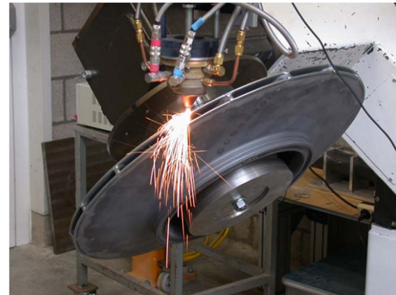
Turbine wheels repair (Rombouts et al, 2006)
