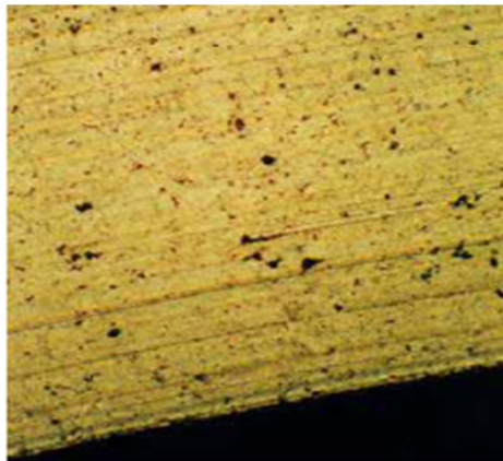
Carbon Ring - LST Seal After 550 Hours
