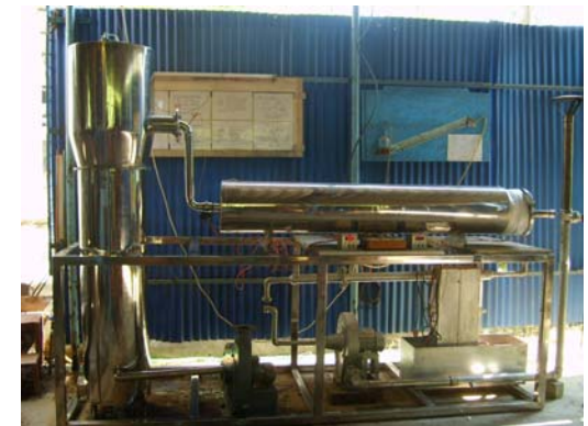
Updraft gasifier with catalytic cracker
