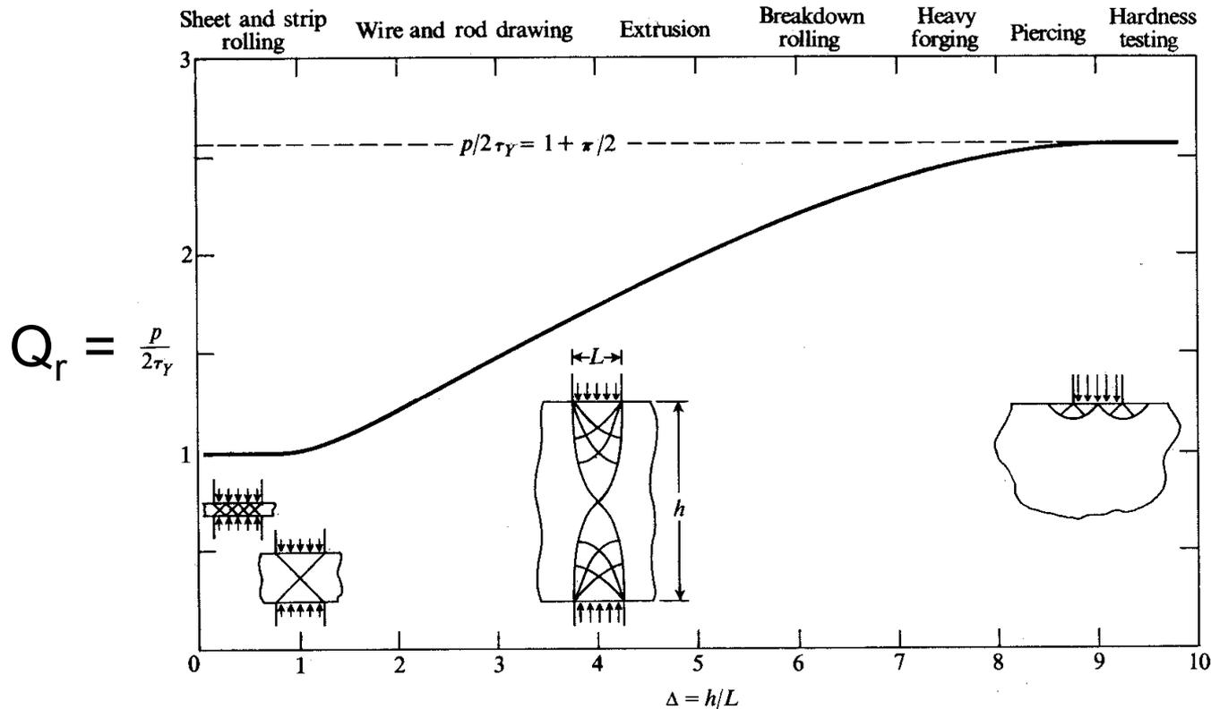
Fig. 7-1. The  $\Delta$ -dependence of yield pressure for the frictionless plane strain-indentation of a nonstrain-hardening material.
