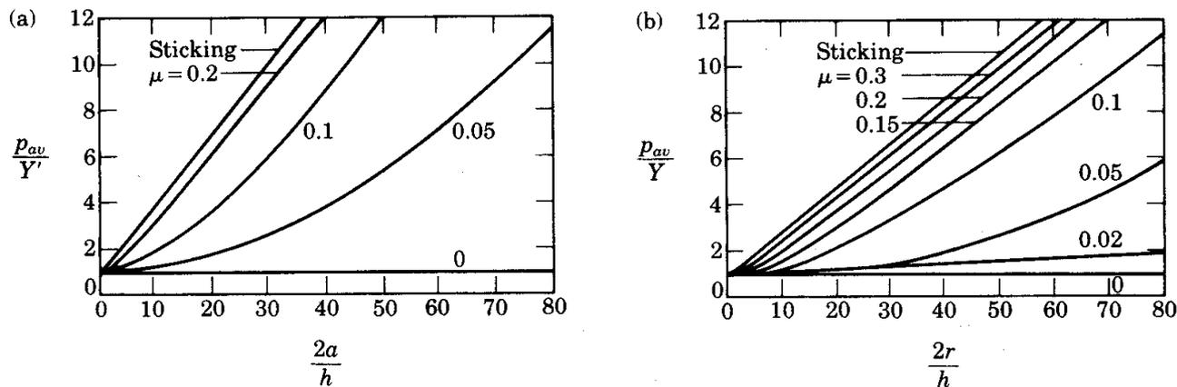
**FIGURE 6.9** Ratio of average die pressure to yield stress as a function of friction and aspect ratio of the specimen: (a) plane-strain compression; and (b) compression of a solid cylindrical specimen. Note that the yield stress in (b) is  $Y$ , and not  $Y'$  as in plane-strain compression in (a).
