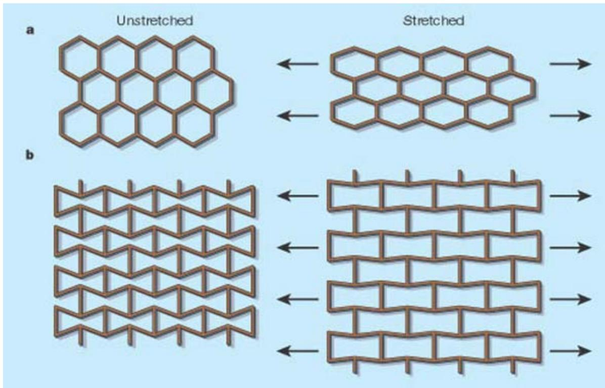
Stretching these two-dimensional hexagonal structures horizontally reveals the physical origin of Poisson's ratio. **a**, The cells of regular honeycomb or hexagonal crystals elongate and narrow when stretched, causing lateral contraction and so a positive Poisson's ratio. **b**, In artificial honeycomb with inverted cells, the structural elements unfold, causing lateral expansion and a negative Poisson's ratio.
