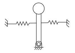
Question 7 : A 100 kg mass undergoes damped vibrations. The spring constant is 100 N/m. The ratio of damping coefficient to critical damping coefficient is 0.1. What is the damped natural frequency? If the initial amplitude of oscillation is 10 mm, what will the amplitude be after 3 oscillations?
