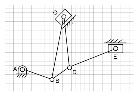
Question 5 : Obtain the acceleration of E of question 6 by graphical method.(You will be judged primarily by the method of graphical construction. Accuracy of drawing carries low weightage.)
