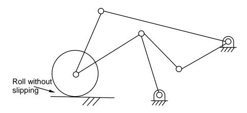
Question 4 : The mechanism shown below has been drawn on a 5mmX5mm grid. The link AB rotates about A at 20 rpm in the clockwise direction. Obtain the velocity of E by graphical technique. (You will be judged primarily by the method of graphical construction. Accuracy of drawing carries low weightage.)
