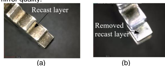
Fig. 5. Steel gear workpiece (a) before and (b) after finishing
