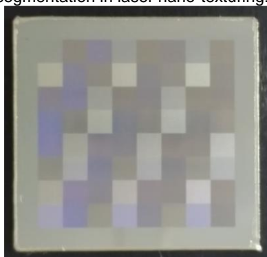
Figure 4. Nano-textured panel with 8 x 8 segments identified by the different surface-plasmonic reflection.
