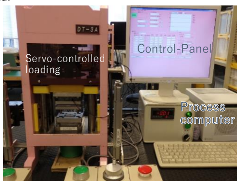
Figure 3. CNC-stamping system for fine piercing under nearly zero-clearance between punch and die.
