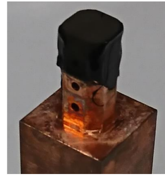
Figure 13. A heating copper block with the micro-textured Fe-Ni layer on its head.
